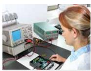
Connection of displays and first quality check of impulse output frequencies
